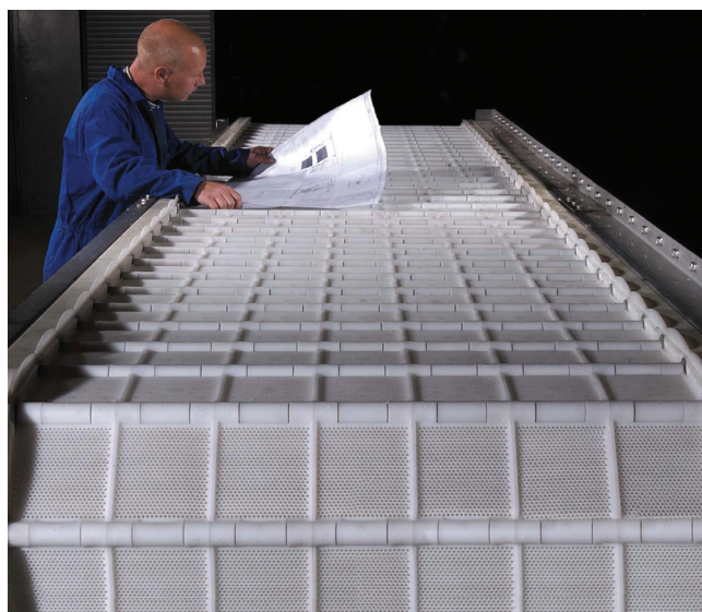
Band Screens under construction
