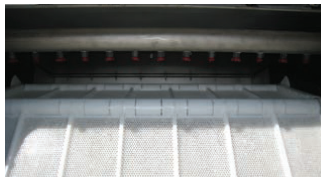
Patented mesh panels eliminate the problem of hairpinning and blinding found with other band screens
