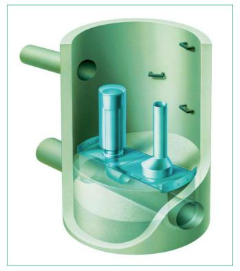
The 'HydroFlush®' is a device that can be installed in chamber connected to the problematic sewer section. A water feed is provided which either 'drip feeds' or fills the 'flushing chamber' at a pre-determined frequency. When reaching the designed level, the flusher unit allows the water to empty into the sewer providing a self-cleansing flow along the sewer to mobilise settled
