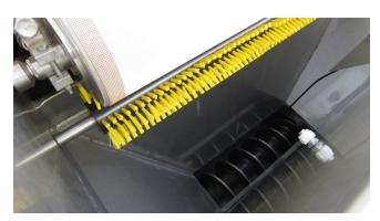
Cleaning the belt with a brush and water is one of the most energy efficient solutions. It prevents the spreading of particles and bacteria through the air. This, combined with its low noise level, gives your staff a good working environment.
