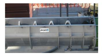
The 9mm thick perforated mild steel trough incorporates 6mm diameter, tapered holes for efficient fluid discharge.
