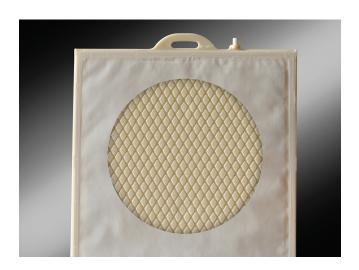
The panels have a pore diameter of less than 0.1µm and provide an excellent effluent turbidity of under 5mg/I SS or less than 0.1NTU. The membrane also has excellent flux characteristics, with pure water permeability (PWP) flow rates of 0.4m³/m²/day to 0.6m³/m²/day.
