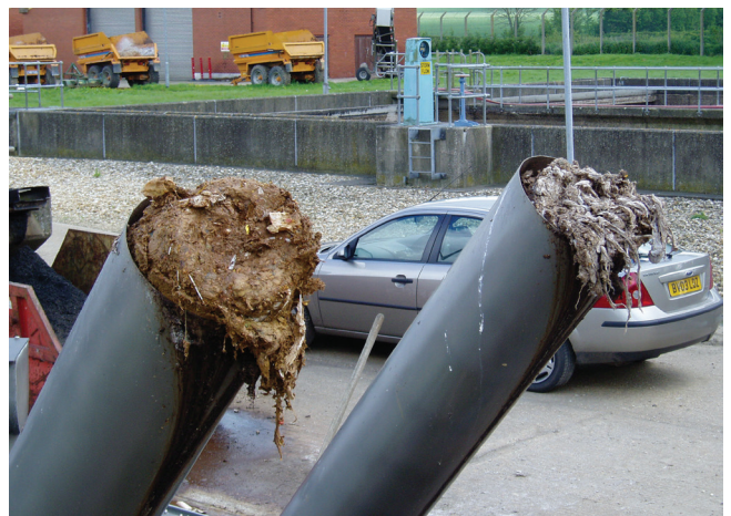
Before and after pictures of the J+A Washpactor-Jet™ machine that has been fitted with the wash water feature. This feature is an integral part of the J+A Washpactor-Jet™ design. The improvements (both visually and in terms of odour) are significant and sufficient for normal conditions.
